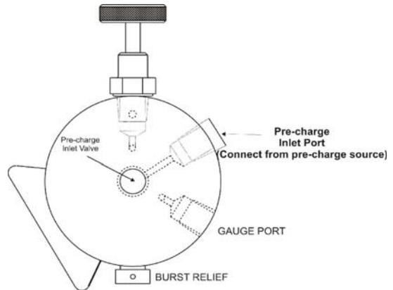
Figure - 3 Pre-Charge End Cap Detail
