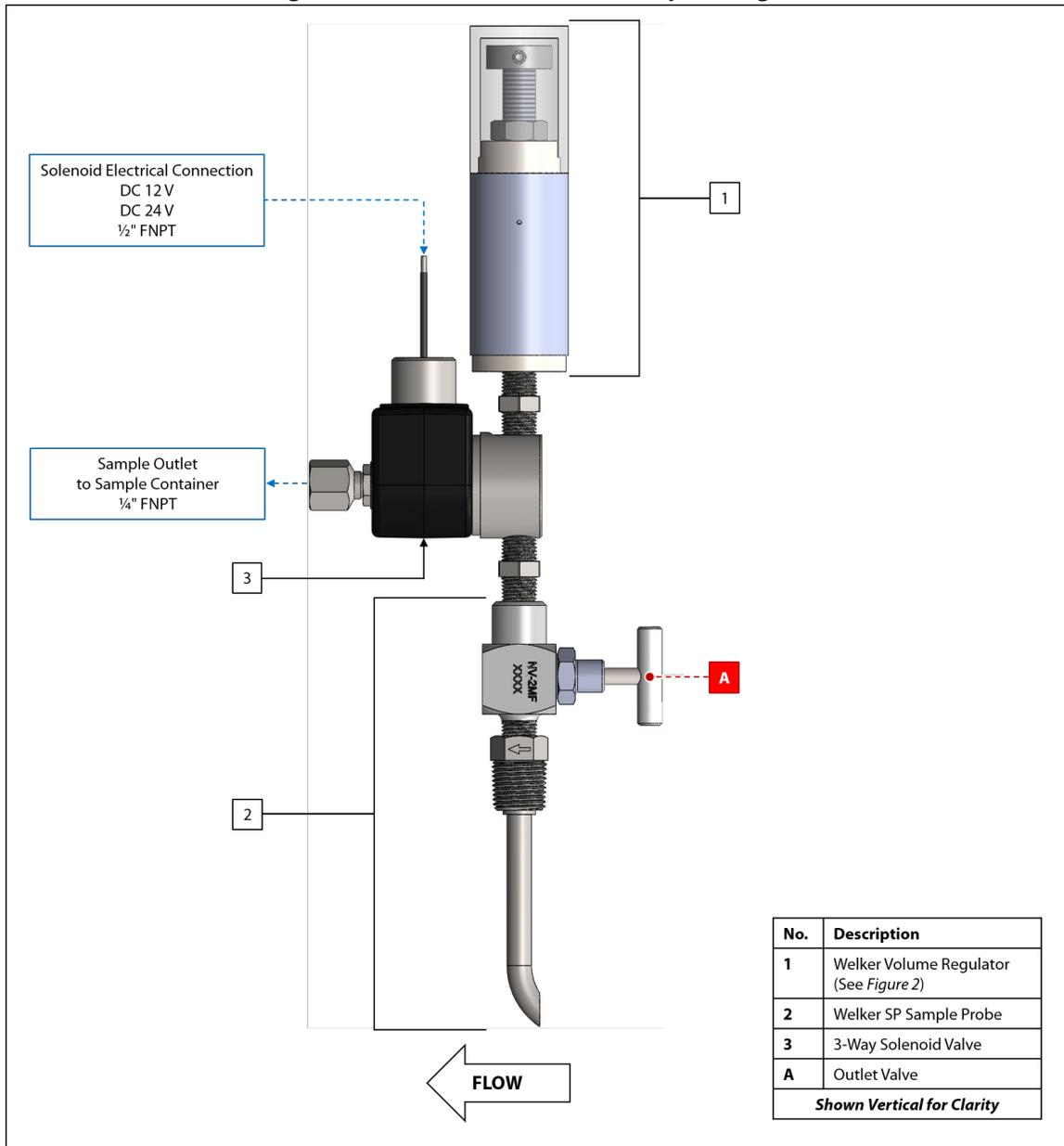
**Figure 2: Welker Volume Regulator Diagram**
