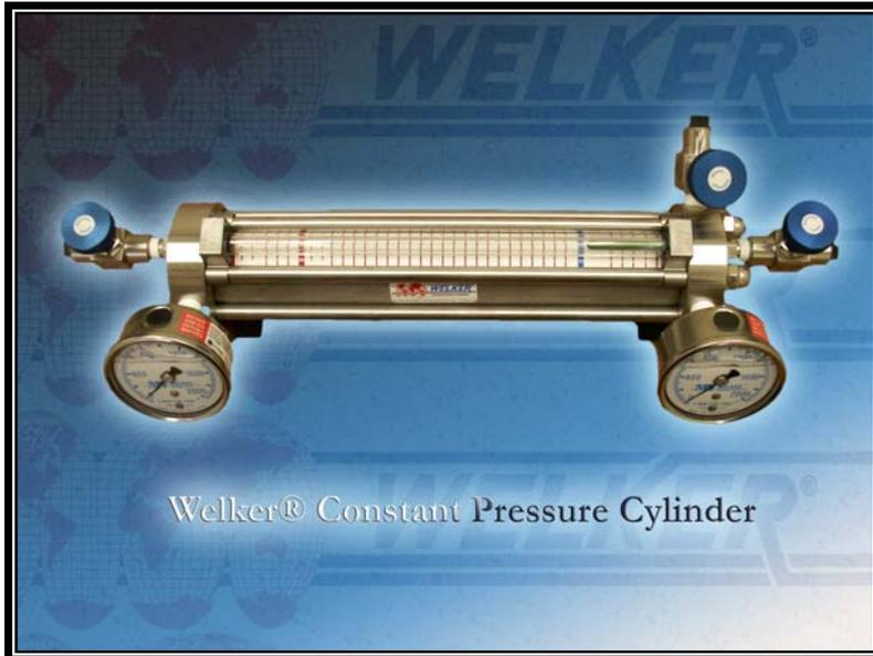
The Constant Pressure Sample Cylinder is designed for use in systems where it is necessary to extract and isolate accurate product samples by maintaining a steady pressure from the pipeline to the cylinder. The cylinders are equipped with a magnetic indicator and a graduated scale set to specify the capacity of the device. During continuous sampling, when the magnetic indicator reaches the 80% mark, all sampling should be stopped. A pneumatic supply pre-charges the cylinder with pressure to
