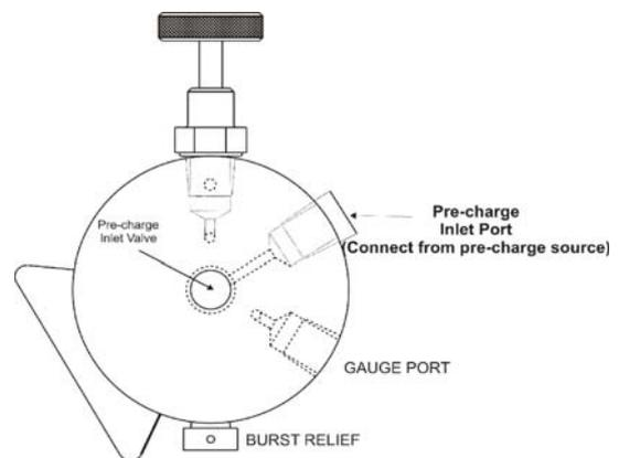
Figure - 3 Pre-Charge End Cap Detail
