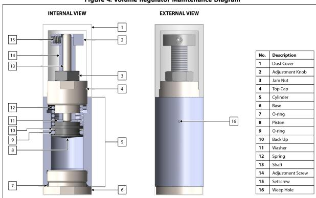
Figure 4: Volume Regulator Maintenance Diagram
