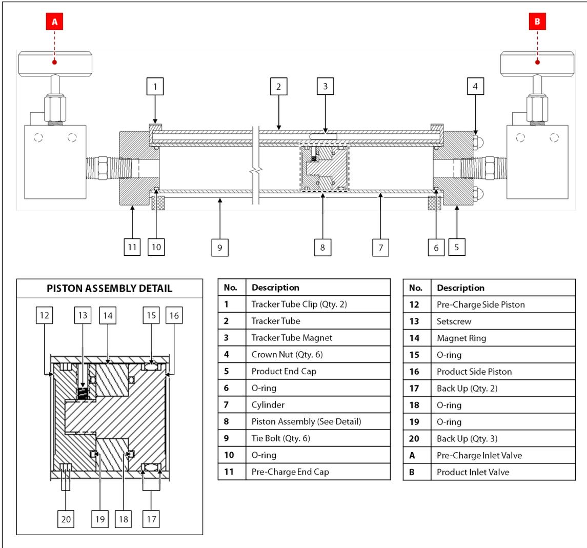
3. Remove the valves and pressure gauges from the end caps.
